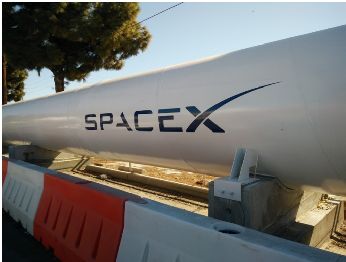
Figure 5 The second largest vacuum chamber in the world, the SpaceX Hyperloop test track used to test vehicles in Competition 1
