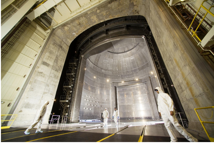
Figure 4 The largest vacuum chamber in the world, NASA's Space Simulation Vacuum Chamber
