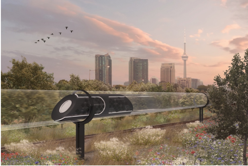
Figure 27 Daytime view of the Waterloo Goose X passing Toronto – clear tubes would only be used at low speeds within the city, closer to 1 atmospheric pressure, rather than the near vacuum state that would necessitate a steel tube.
