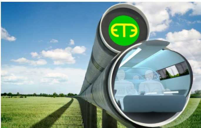
Figure 6 Track proposal by ET3 with a vacuum state 1,000 times less dense than the SpaceX track. Note the large obstruction to track sectional area.
